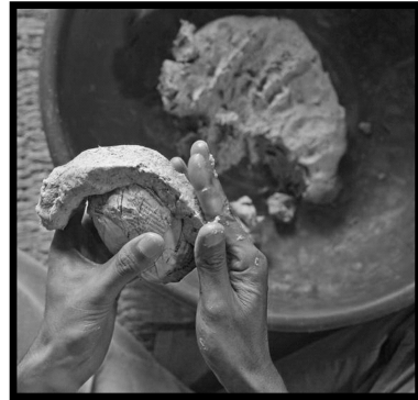
Figure 4: Applying the mashed paper on the mould
